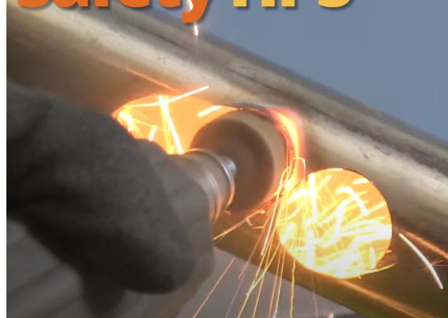
Maximum Safe operating speed of all Mounted points is 33 m/sec. Max RPM is shown for each shape code in the table. Max RPM is based on the shape and Spindle combination with a maximum 25 mm overhang.
